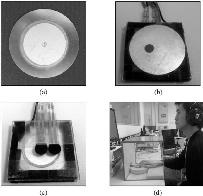
**Fig. 1.** (a) One side of the piezoelectric actuator showing both the ceramic and metal disks. (b) Top view of one stimulator key. (c) Bottom view of one stimulator key. (d) Experimental setup without the visual covers.
