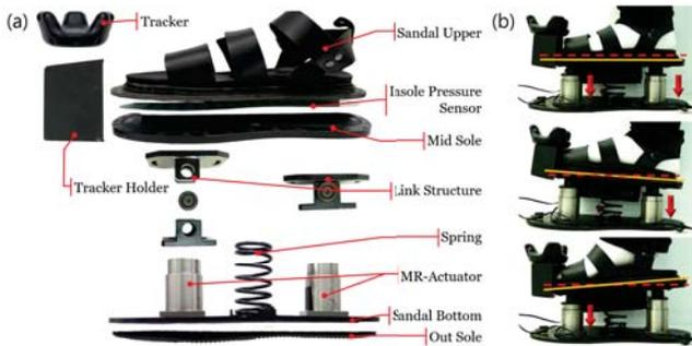
Fig. 2. Structure of RealWalk. (a) Exploded view and (b) Link structure and its motions
